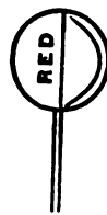
Stop signal for the line to which the Red Signal is turned.
